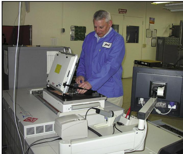
Test Manager David Perry prepares a circuit board for testing.
